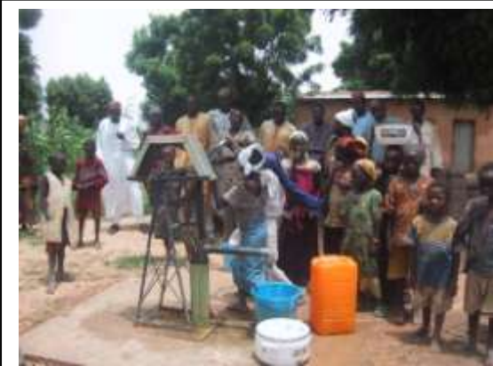
At 16m to water it takes two children to raise the water easily with the rope pump.
