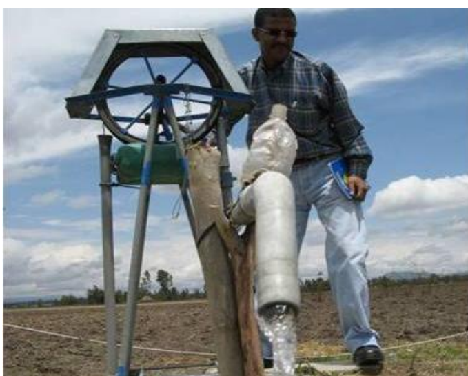
Figure 5: Rope Pump for Domestic and Irrigation Use
