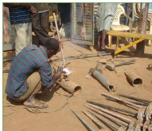
Construction of Drilling Tools
